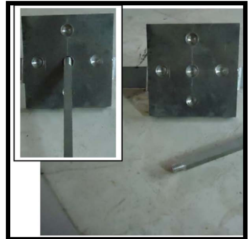
Plate (2): Square Aluminum Raft Model, Piles and the Screwed Opening to Fix Piles.
